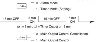
If 'MOC' is 1 then Timer is ON as Main Output is automatically OFF. When using MOC function, you can effectively use Timer Output as Defrosting Function.
